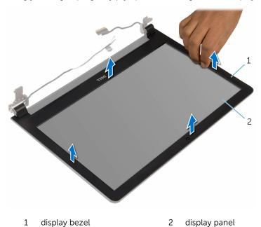
2 Lift the display bezel off the display assembly.
