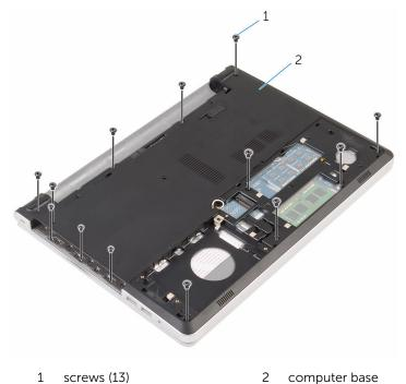
5 Using a plastic scribe, pry up the computer base from the palm-rest assembly, starting from the area around the display hinges.
